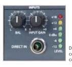
Direct input. Fontal and rear connection. Gain and balance controls.
