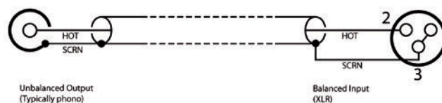
Fig. 03: Balanced to Unbalanced Analogue wiring and PIN out.
